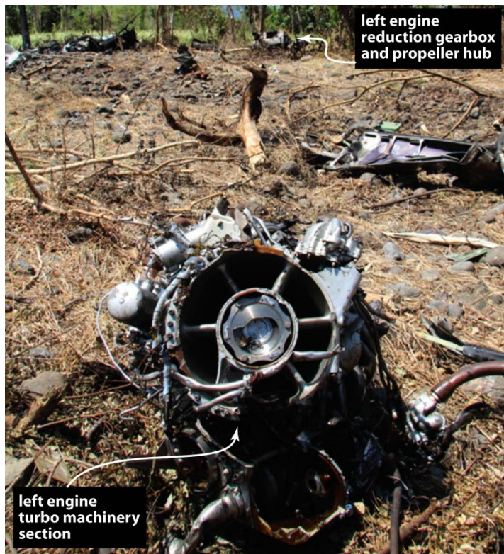
Figure 4: Left engine (after sectioning at the accident site)
